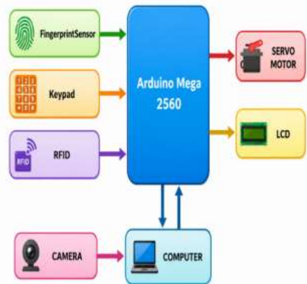
FIGURE 4. Operational flowchart of the proposed smart door lock authentication algorithm.
