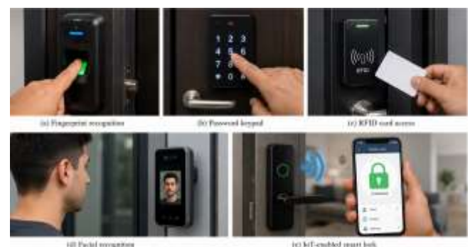
FIGURE 1. Representative smart door lock authentication technologies: (a) fingerprint recognition, (b) password keypad, (c) RFID card access, (d) facial recognition, and (e) IoT-enabled smart lock.
