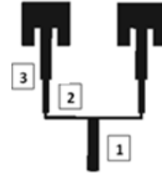
Fig 6. Proposed 1x2 array geometry microstrip antenna.
